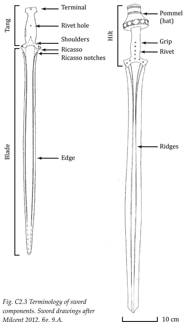
Fig. C2.3 Terminology of sword components. Sword drawings after Milcent 2012, fig. 9.A.
