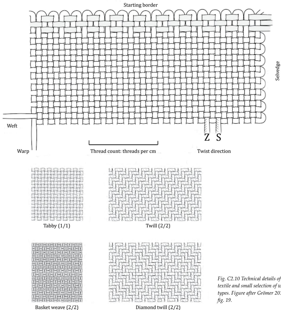
Fig. C2.10 Technical details of a textile and small selection of weave types. Figure after Grömer 2013, fig. 19.
