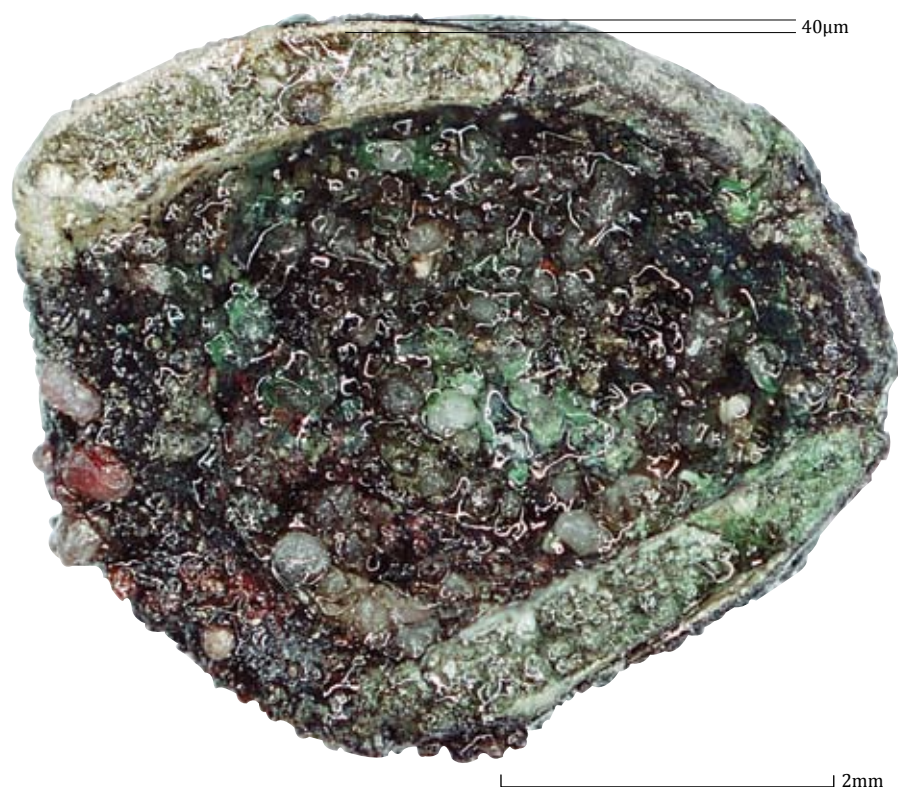
Fig. 9.3 A look at the inside of the head of a stud. Due to fracture of the legs, the cross-section shows a white outer layer of about 40 µm thick. Also, grain-like green and red products can be seen. Figure by J. Nienhuis/J. van Donkersgoed.
