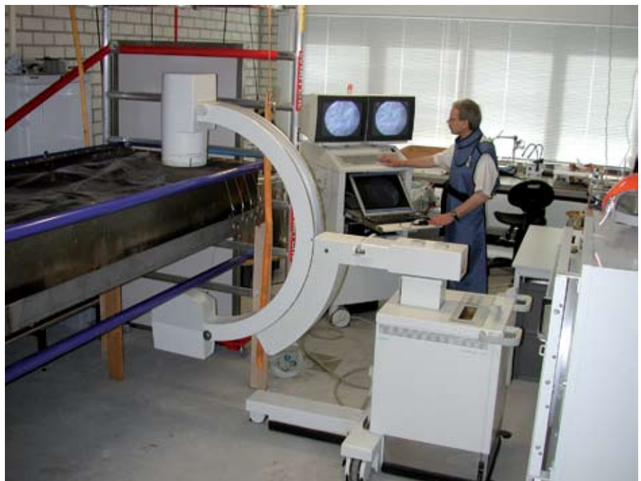
Fig. 8.9 V 1003 suspended in a frame whereby the X-rays are taken using a C-arm. Figure by Restauratieatelier Restaura, Haelen.
